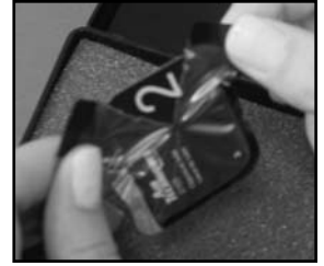
Figure 4 Ejecting a Plate into the Plate Transfer Box
